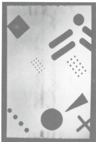
Fig. 10. Laminogram of copper/steel phantom; processing time was 10 minutes.
