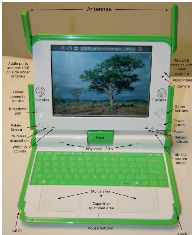
Figure 1. Diagram of the XO laptop [6]
